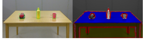
Figure 1: Illustration of the used objects and the corresponding 3D point cloud information: (A) car, (B) bottle, and (C) cup.
