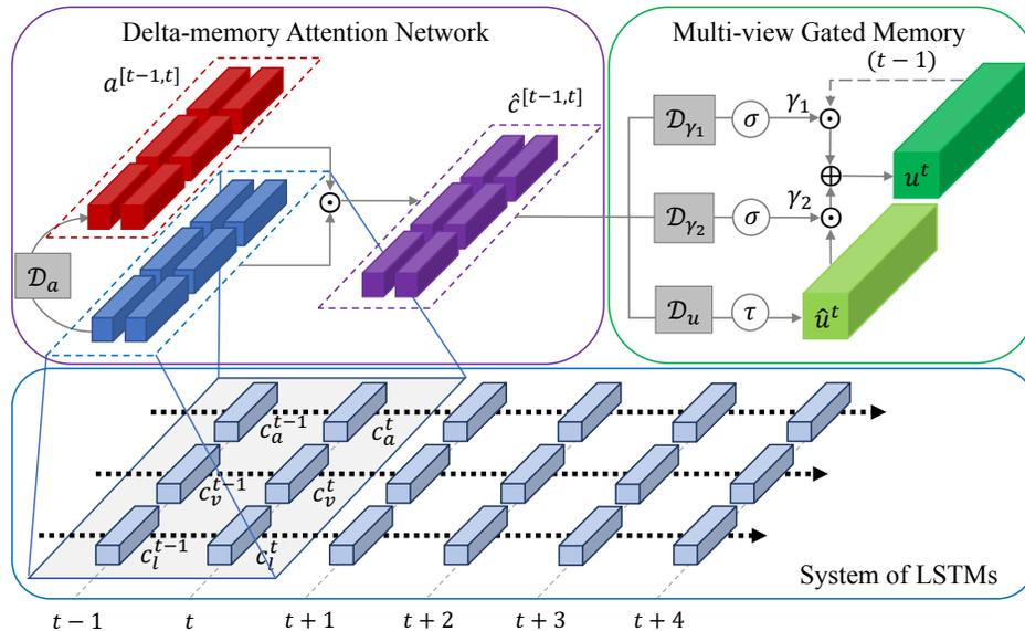
Figure 1: Overview figure of Memory Fusion Network (MFN) pipeline.  $\sigma$  denotes the *sigmoid* activation function,  $\tau$  the *tanh* activation function,  $\odot$  the Hadamard product and  $\oplus$  element wise addition. Each LSTM encodes information from one view such as language ( $l$ ), video ( $v$ ) or audio ( $a$ ).
